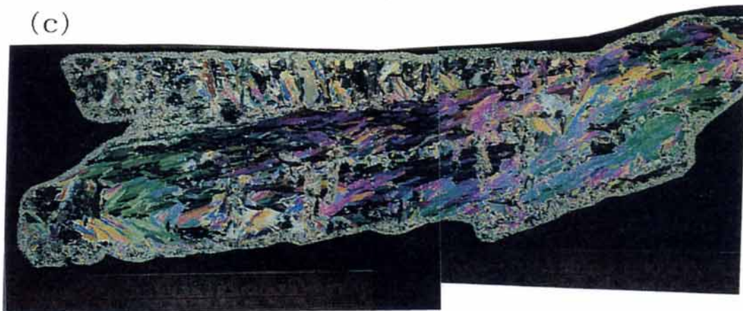
Figure 5.3.12 Vertical structure of pancake ice P3 (1997)
